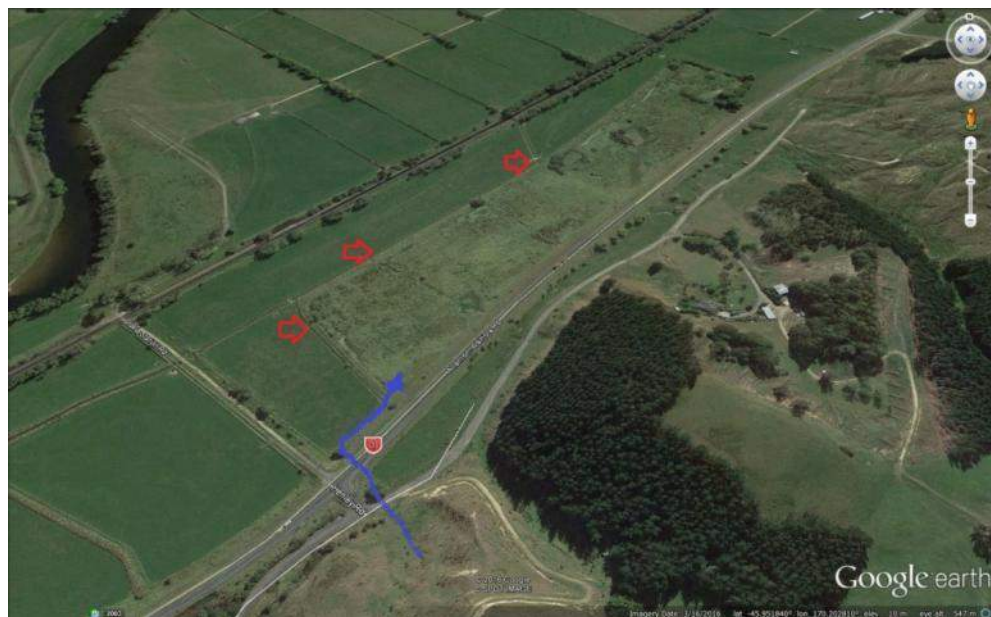
Figure 13: Aerial view of the Otokia Wetland showing perimeter drainage (red arrows). The blue line is a small water catchment that could potentially be diverted into the wetland.
